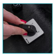
If you have a duo machine, select the speed you wish to operate at. Always ensure the machine is switched off before changing the speed setting.
