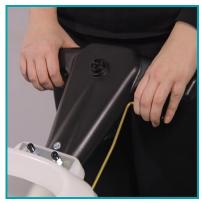
The flow of solution from the tank is controlled by moving the left hand lever. Releasing the lever stops the solution. Proceed to operate the machine in the normal manner, releasing solution as required.
