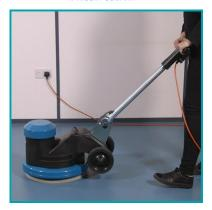
The normal movement of the machine is from side to side across the floor. Whilst it is engaged in the normal working position, lower the handle to move the machine to the left. Raise the handle to move the machine to the right.
