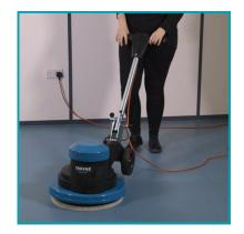
Adjust the handle to a comfortable working position using the handle lever.
