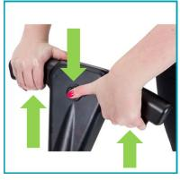
Push the power button and then press and hold the switch triggers to start the machine. The switch triggers must be held whilst using the machine.
