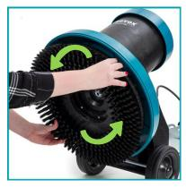
Fit the brush or drive board and pad onto the drive plate and rotate it anti-clockwise until secure.
