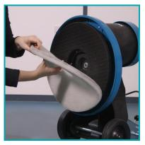
Remove the brush or drive board & pad. Never store the machine with a brush or drive board and pad fitted as this can cause distortion, and results in instability during operation.
