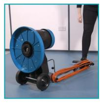
Pull the handle down until it rests on the floor and the brush guard is raised.
